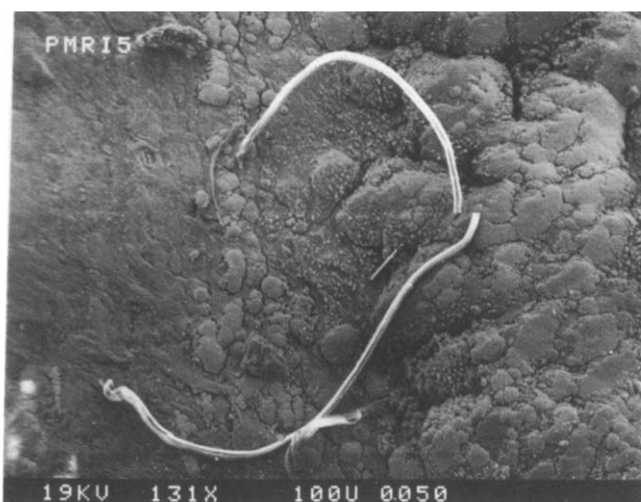
Figure 4 Scales of deposits on a PMR-15 specimen showing strands of cotton contaminant
